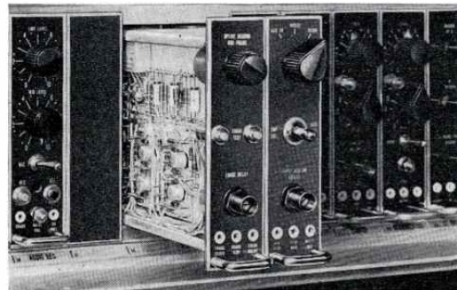
FIG. 9. Electronic splicing and editing accessory provides means for adding or inserting program segments.
