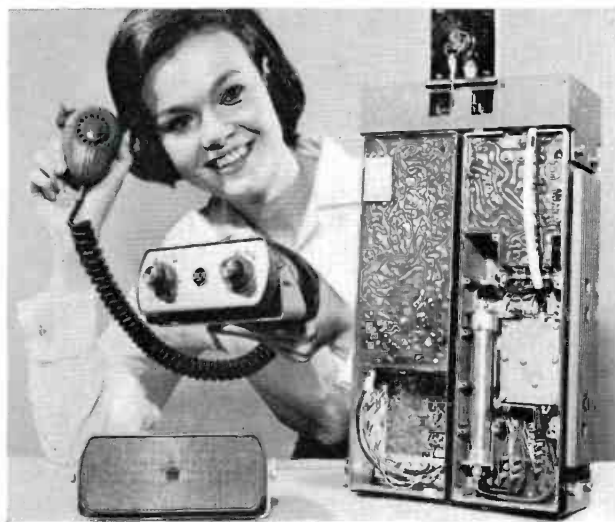
FIG. 3. Show-off Gloria Kirby displays new solid-state radio unit. Note clean, simplified circuitry design of Super-Fleetfone. Cylindrical component at bottom of transmitter chassis is self-powered solid-state antenna switch.
