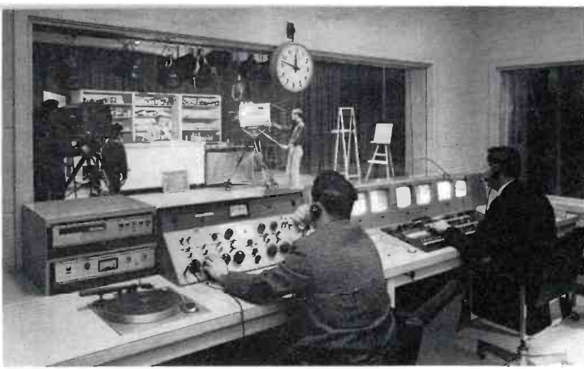
PRODUCTION CONTROL CENTER designed by station technical staff using RCA "New Look" equipment. Personnel monitor audio and video; perform switching to record programs on television tape. Equipment (L to R) consists of RT-7 Cartridge Tape (and turntable), BC-8 Audio Console, TS-40 Program Switcher.
