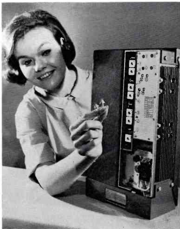
FIG. 3. Show-off Gloria Kirby displays new solid-state radio unit. Note clean, simplified circuitry design of Super-Fleetfone. Cylindrical component at bottom of transmitter chassis is self-powered solid-state antenna switch.
