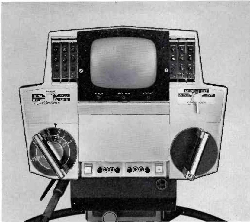
FIG. 2. Rear of camera showing large "D" handles for zoom and focus control. Handles can also be used to maneuver camera. Viewfinder is large 8-inch type. Plug-in modules are easily accessible.
