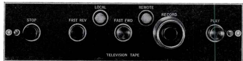
FIG. 10. Remote control panel permits remote operation of recorder/player.
