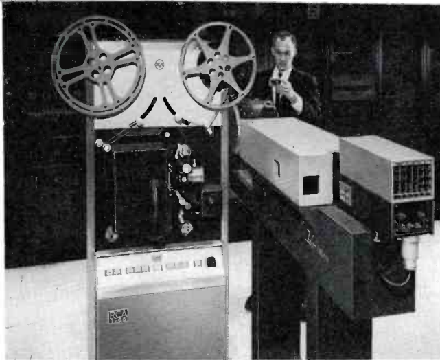
NEW TELEVISION FILM SYSTEM handles 35mm slides and 16mm motion pictures for use by ETV instructors in their prepared presentations. Equipment includes TP-66 Film Projector, TP-7 Slide Projector, TP-11 Multiplexer, TK-22 Film Camera. This new camera operates without adjustment throughout the entire day.
