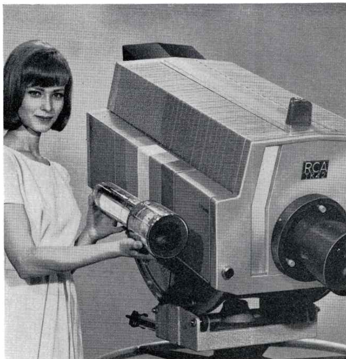
FIG. 1. TK-42 live color camera employs large 4½-inch I.O. luminance tube for superior pictures in color and black and white.
